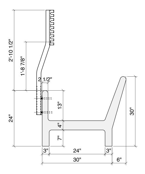
Advantages: Sloped Back Saves Feed Rounded Top Rails Portable - Can Be Moved Rodent Proof - Ends Are Sealed
